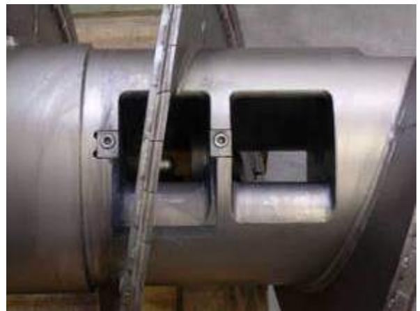
The bowl is equipped with stainless steel strips to secure against abrasion. The solids discharge area of the casing is protected with wear liners of stainless steel.
