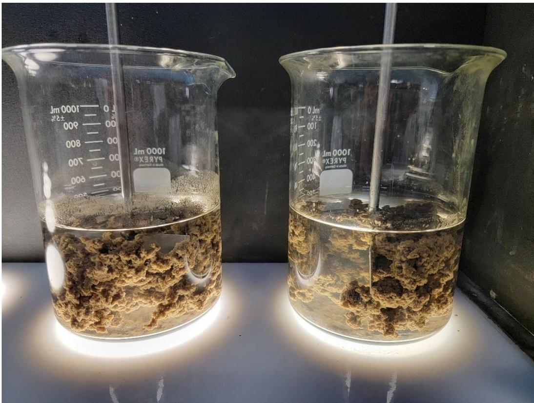
**Figure 2:** Optimal floc observed at a polymer dose of 7.5 lbs/ton of K279 (left) and K275 (right)
